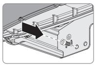
11. Ensure that the inverter is securely in place.
