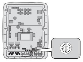
Figure 12: Positions of rotary switch C
